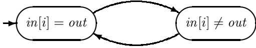
Fig. 6. Another predicate-action diagram of \langle in[i], out \rangle for \Pi_C , where 1 \leq i \leq n .
